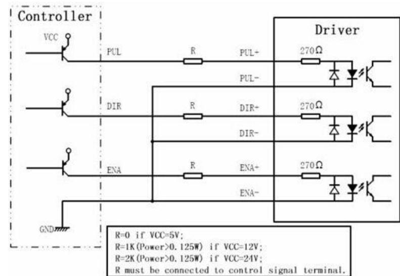
Figure 3: Connection to PNP signal (common-cathode)
