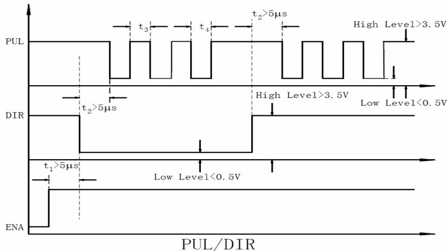
Figure 5: Sequence chart of control signals
